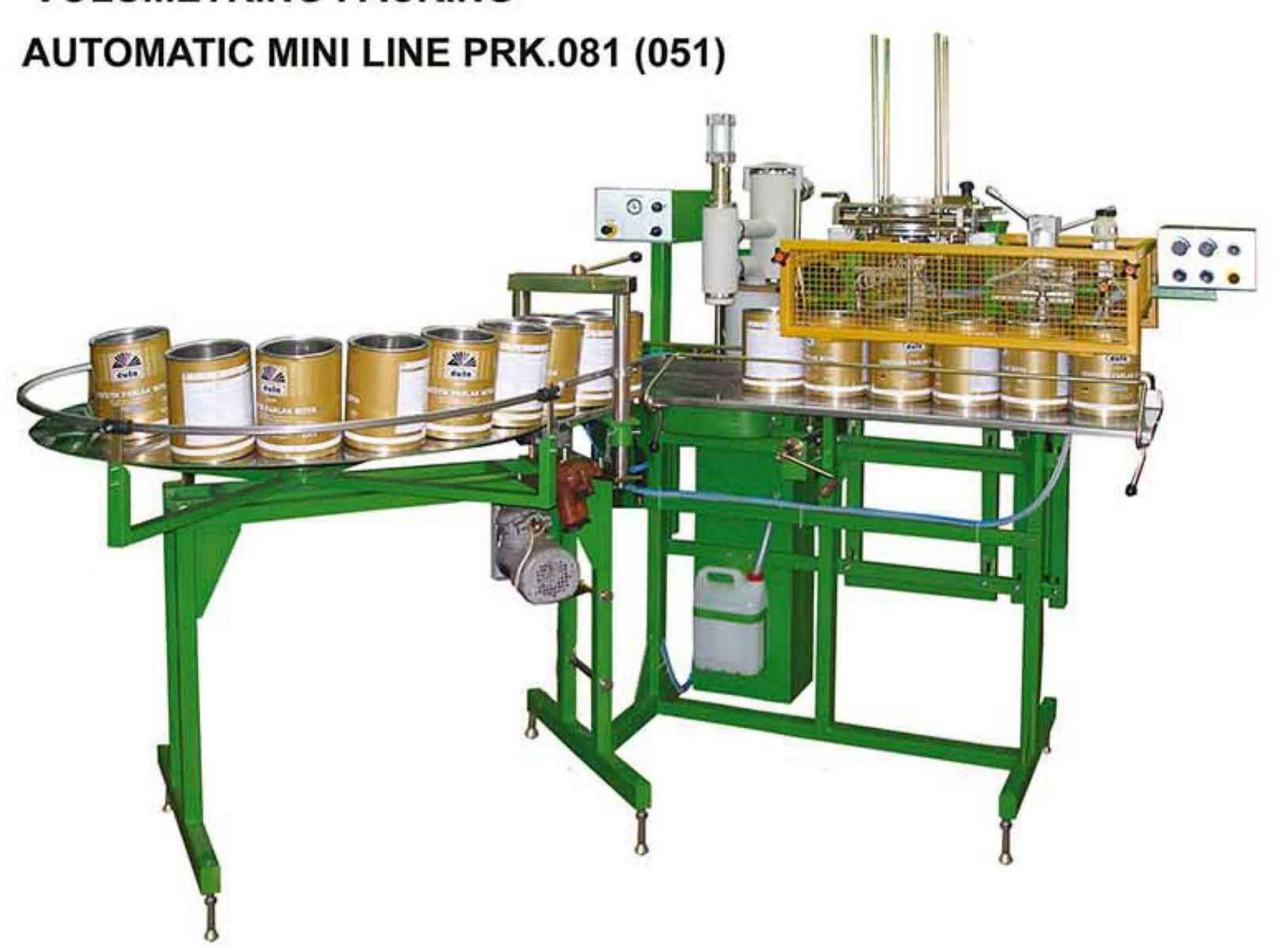
For dosing products of low and medium viscosity, from 0,25l to 5l
